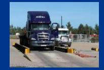
2 x 22m Weighbridge (Capacity: 70 Tons) 1 x Group Axle Scale
